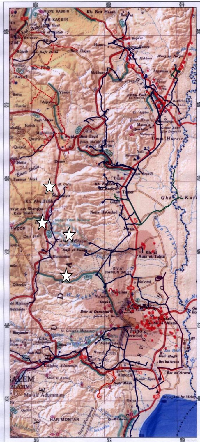
Figure 1: Location map of new sites for brackish water wells (stars) implemented on well (black circles) and pipe line black lines) location map of Mekorot.
