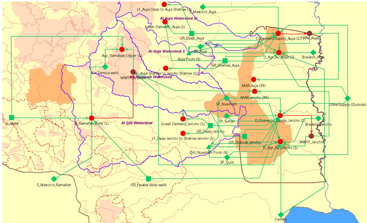
**Figure 6.1:** Schematic of the existing water resources system at Cluster West together with the potential “Upgrades” as basis for the application of the WEAP model
